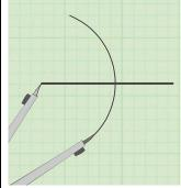
Put the point in the other end and draw an arc from that point, crossing the first arc in two places.
