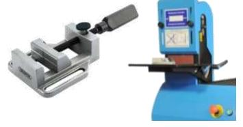
Machine vice -Used to hold workpiece securely sand/smooth during drilling.
