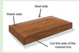
When cutting from a long length of wood we should always mark one first, cut to length on the waste side of the line allowing for the kerf of the saw. Then mark the second section and repeat the process.
