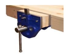
**Wood Vice** – Used to secure material while working on it (cutting, filing sanding etc.)
