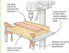
A jig is a device used to hold a piece of material and guide tools. They are used to ensure the process can be repeated accurately and to a high quality.
