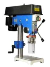
Pillar/Bench Drill – Used to drill holes into different materials.
