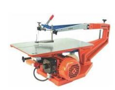
Scroll-Saw/Hegner-Saw-Used to cut complicated shapes in thin material.
