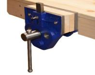
Wood Vice – Used to secure material while working on it (cutting, filing sanding etc.)
