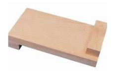
**Bench hook** – Used to hold work in place when cutting
