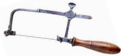
Piercing Saw – Used to cut thin sheet metal.
