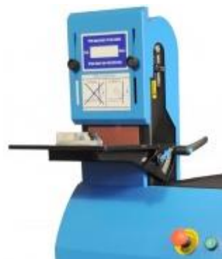
Band facer/Belt Sander Used to sand rough material smooth.
